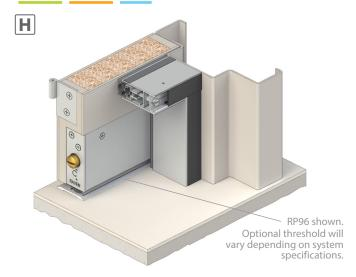
Perimeter seal adjustment independent of fixings
