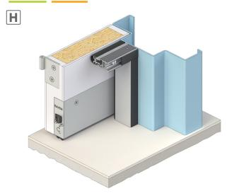
Perimeter seal adjustment independent of fixings
